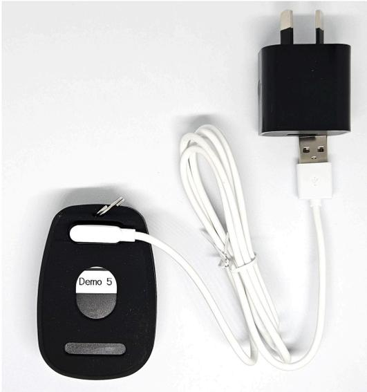
Figure 1. Using the magnetic charging lead
